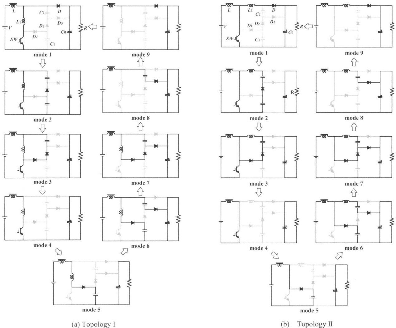
Fig. 3. The operating modes of soft switching PWM boost chopper-fed DC-DC converters.
